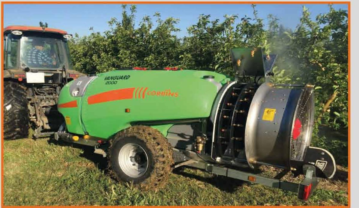
**HELIX:** Diameter 920 mm, variable blades and progressive step in 8 positions (25 ° to 45 °). Type SICKLE fdv reinforced polyamide, low power consumption and high performance. Centrifugal clutch in 3 brake shoes.
